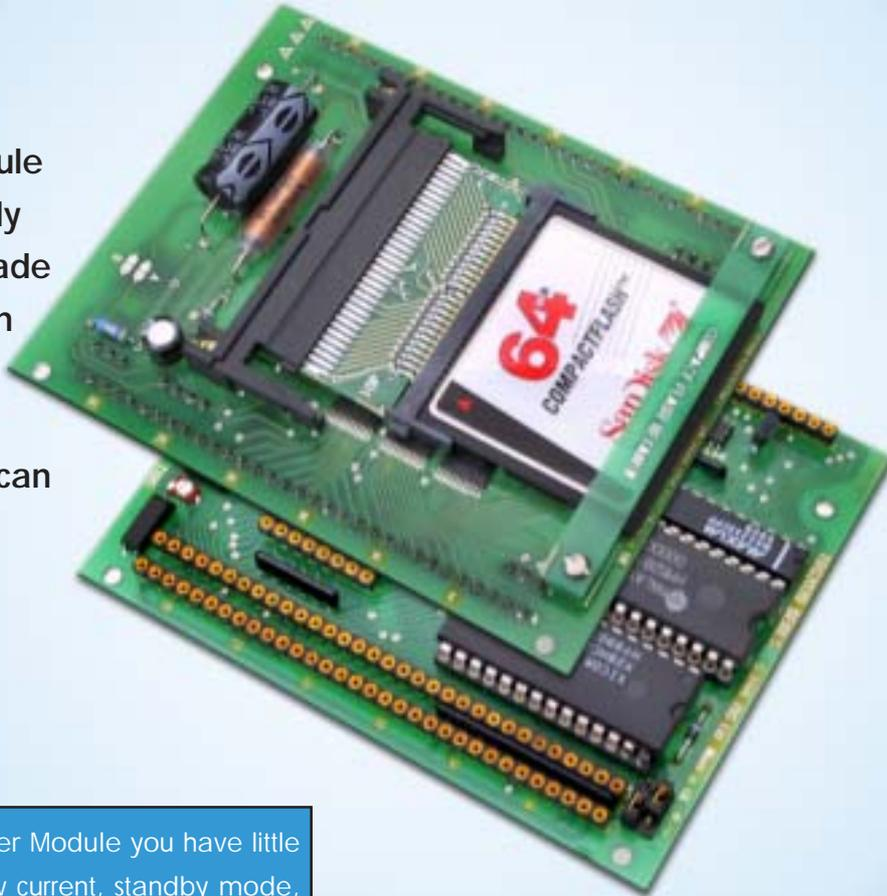
As a Data Logger Module you have little to add to its low current, standby mode, over a gigabyte of memory, 10-bit 8-channel A to D and real-time clock. There are keyboard, graphics LCD, CAN and serial port interfaces. Use Industry standard digital camera Compact Flash and PCMCIA-ATA cards. You can also log to a flash chip on the computer.
